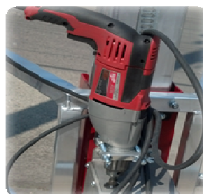
4 - Power the lift with your drill
